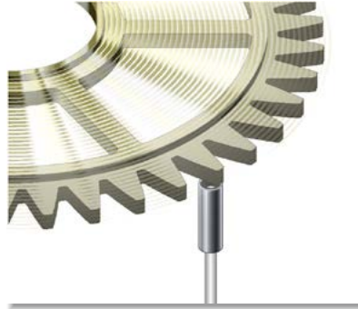
Detecting rotation of a gear
