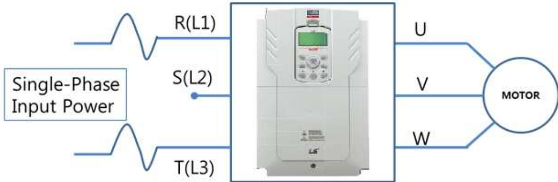
Figure-3 Terminal Wiring Diagram
